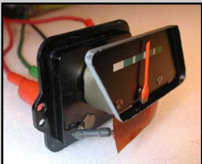
12V Fuel gauge showing deflection under 12V power, 100 Ohms simulated sender R. Visible is gray 82 Ohm input resistor.
