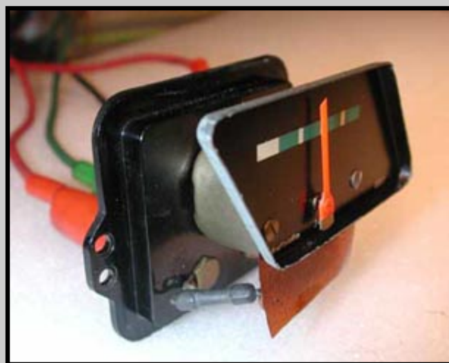
Only slight decrease in deflection is noted after operating voltage is decreased to 6V.
